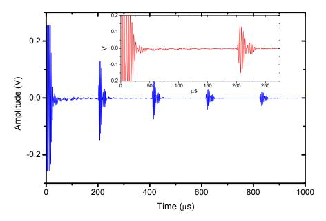
The highest sensitivity is obtained when the piezocomposite disk acts as transmitter and receiver, that is, the ferroelectret film is used a conventional passive matching layer. On the other hand, when the ferroelectret film is used as both transmitter and receiver the sensitivity is about 30 dB below. Bandwidth is similar for the three cases.
