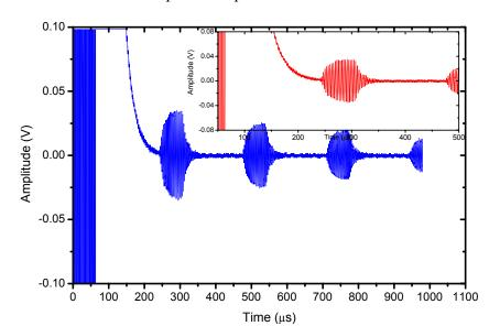
**Figure 14.** Pulse-Echo with the piezocomposite disk. Tone burst excitation at 315 kHz.
