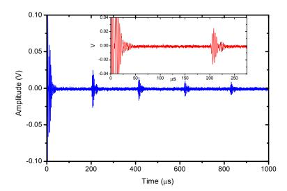
Figure 12. Pulse-Echo (transmit and receive) with the ferroelectret film.
