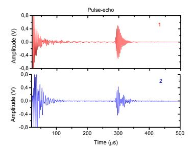
**Figure 17.** Sensitivity in pulse-echo mode of operation wideband excitation (spike). 1. (Red) Air-coupled transducer with active matching layer. 2. (Blue) Conventional air-coupled transducer with passive matching layers.
