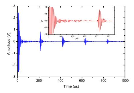
**Figure 11.** Pitch-catch response. Transmitter: 1–3 connectivity piezocomposite, Receiver: ferroelectret film.
