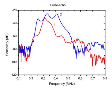
**Figure 18.** Pulse-Echo mode of operation, narrow band excitation (tone burst). Conventional air-coupled transducer with passive matching layers (compare with Figures 13 and 14). Reflector at 45 mm.
