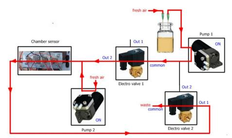
Figure 3. Flow of gases at the injection stage.
