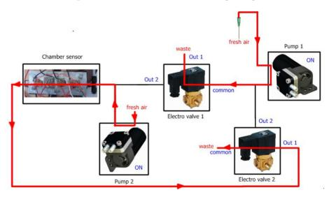
Figure 5. Flow of gases at the cleaning2 stage.
