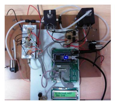
Figure 2. View of the mbed electronic nose.
