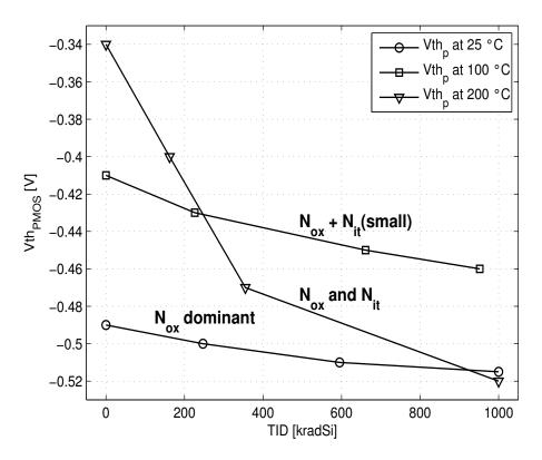
Figure 12. Measured PMOS voltage threshold vs TID at different temperatures.
