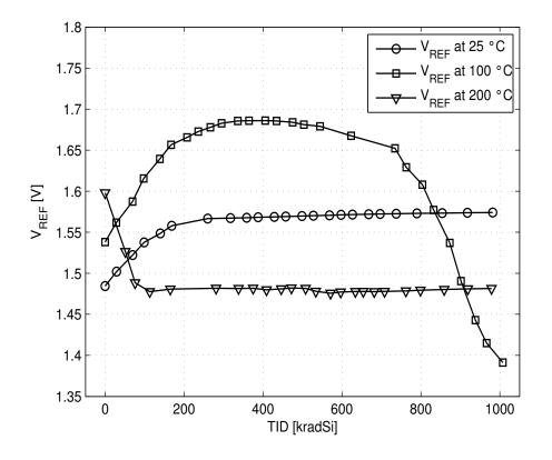
Figure 10. Measured voltage reference  $V_{REF}$  vs TID at different temperatures.
