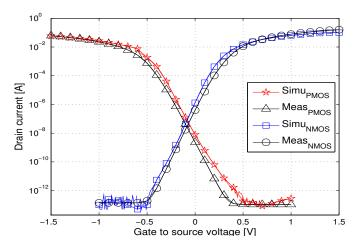
Figure 5. Measured and simulated  $I_D$  versus  $V_{GS}$  curves at 200 °C,  $V_{DS} = 1.5$  V, W = 1  $\mu$ m, L = 0.28  $\mu$ m.
