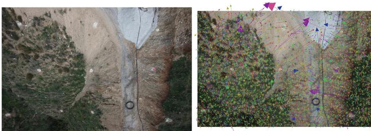
**Figure 12.** Single feature matching (**left**) and the complete set of matchings (**right**) in a given pair of images.
