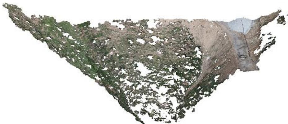
Nevertheless, the computed DSM is defined within its local coordinate system. Therefore, the final step consists of georeferencing the model, *i.e.*, the model coordinates have to be transformed into world coordinates. This can be performed, for instance, by applying Horn's method [39] to compute the optimal affine transformation (rotation  $R$ , translation  $T$  and scaling  $S$ ) that best maps a set of points of the model,  $P^M$ , into the real world,  $P^W$ :
