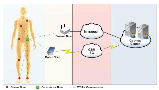
Figure 1. WBAN motion architecture.
