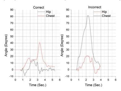
Figure 7. Comparing the data collected during a correct and an incorrect pickup action.
