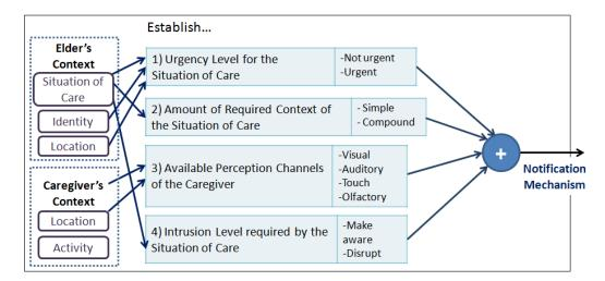
**Figure 4.** Model for the Design and Selection of the notification mechanisms.
