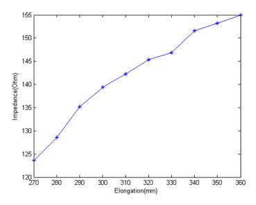
Figure 14. Relationship between impedance and elongation.
