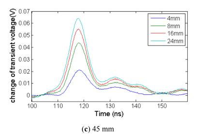
With different deformation section, the waveforms show that the spike magnitude increase when the sensing cable is stretched from 4 mm to 24 mm with different deformation section lengths. It verifies the conclusion which is made according to the theoretical analysis above.
