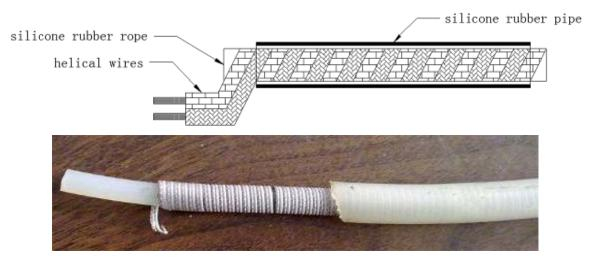
Figure 4. Structure of elastic helical TDR sensing cable.
