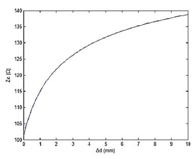
The relationship curve shows that EHTSC's impedance increases when the cable is stretched and the rate decreases when  $\Delta d$  increases. That means EHTSC can effectively detect the deformation in a certain range near  $\Delta d = 0$ .
