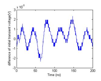
Figure 18. Difference waveform between two initial transient voltage waveforms.
