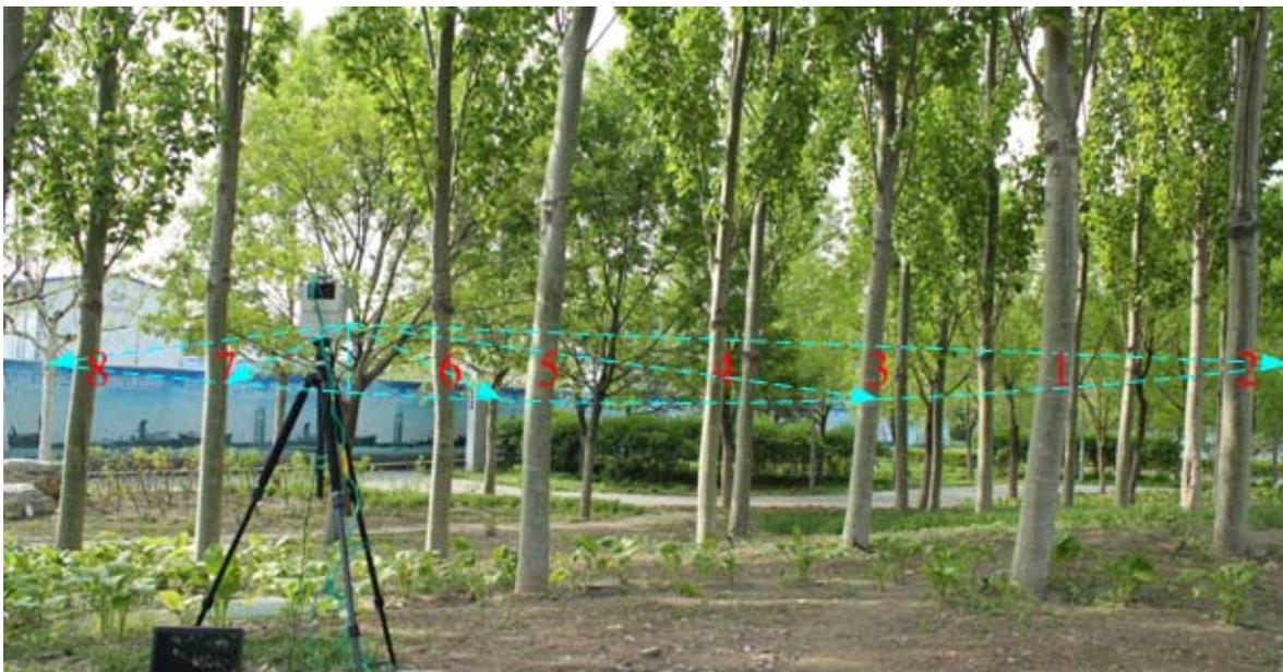
In the experiment, the height of the scanning plane is equal to about 1.3 meters from the ground, this leads to better results because the understory and other uninteresting objects below the scanning plane and the variation in the height of the scanning plane is assumed to be negligible in our experiment. The measurement range is limited to 8 m, which is not beyond the reachable workspace of the crane of the logging harvester and can echo sufficient laser echo data from a single trunk.
