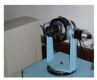
Figure 4. 2D turntable and video camera.
