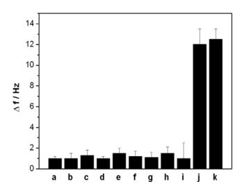
Figure 7. Reusability of the QCM-based  $Hg^{2+}$  sensor challenged with 5 nM  $Hg^{2+}$  and washed with 50 mM cysteine.
