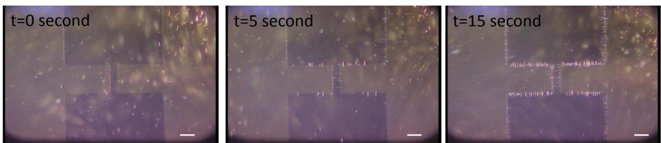
Considering the DEP force and torque, nanowires are attracted to a high electric field region with orientation. More polarizable and longer nanowires can be more easily attracted, which can be used for the selective deposition of nanowires. For demonstration of DEP, 10  $\mu\text{L}$  solution containing Si
