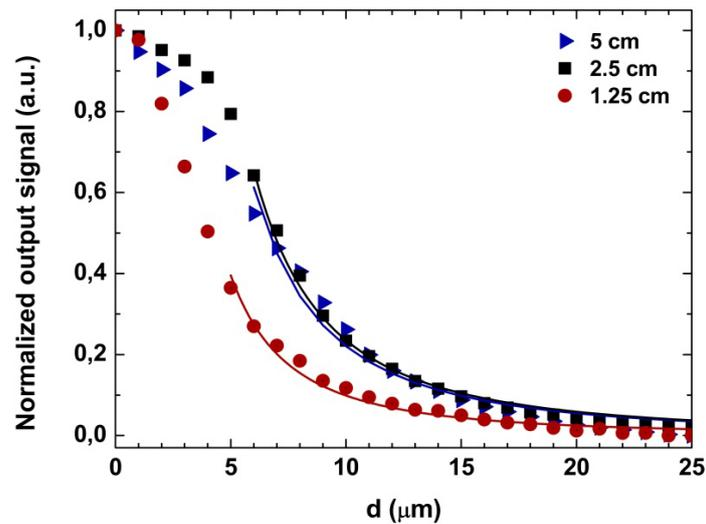
The response of the intensity with the displacement varies in accordance with the inverse square law accordingly with the equation:
