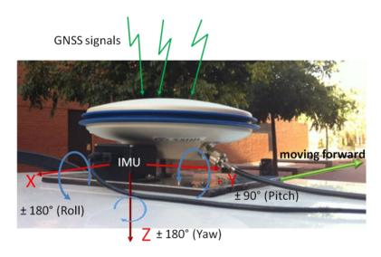
The GNSS receivers that have been selected for base and rover are two NovAtel OEMV-1G boards, which offer GPS + GLONASS L1 tracking and provide reliable positioning even in obstructed sky conditions. The receivers are embedded on a NovAtel compact enclosure (FlexPak-G2-V1G) for outdoor applications as base station and vehicle position in urban environment.
