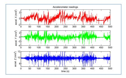
Thus, this sub-module uses the amplitude of accelerometer measures in a window of time (maximum measured value minus minimum) as an indicator of a "flat" reading. The advantages of the proposed method include:
