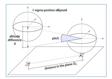
Figure 12. Calculation of elevation angle from two GPS measures.
