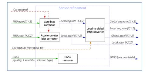
Figure 10. Sensor refinement module.
