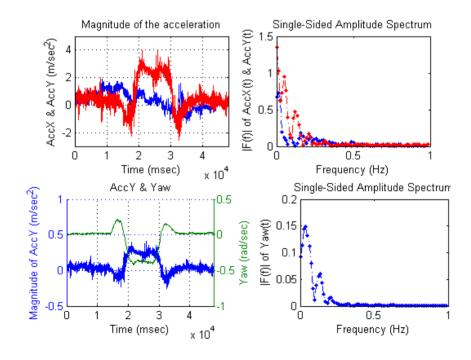
The frequency-domain representation allows us to observe some errors in IMU data, as presented in [46], where Fourier Transform (FT) is used to estimate parameters such as, bias, scale factor, and misalignment of the accelerometers and rate gyros. As an example, the bias component can be found at
