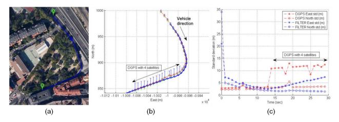
**Figure 22.** (a) Rover trajectory within complex urban canyon. (b) DGPS and GPS solutions (red) and UKF filter solution (blue). (c) Standard deviations of DGPS and GPS: East (upper blue bar) and North (lower green bar).
