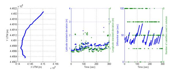
A typical behavior of the receiver in soft urban environment is the commutation between differential mode and GPS SINGLE mode, causing also the corresponding drop of accuracy. This effect can be noticed if the value when differential age is zero.
