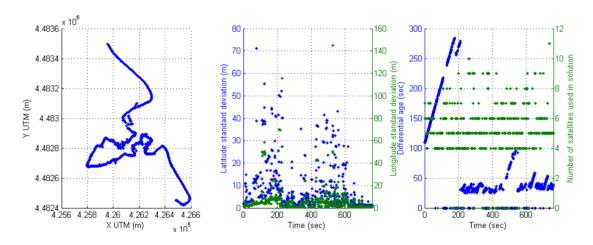
The sensor fusion solution is presented in Figure 20(a), where red trajectory displays the difficult calculation of positioning by rover DGPS system. Inaccuracies are caused by rover navigation within complex urban area. The estimated solution using UKF filter is blue trajectory. The reliability of UKF solution can be observed in detail for 175 s of initial trajectory: Figure 20(b), East coordinate and Figure 20(c), North coordinate.
