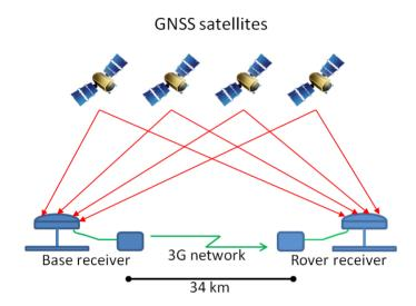
The "optimal conditions" term in SINGLE mode refers to observing six or more healthy satellites and relatively low multi-path (to assure enough quality of the received data). In the case of differential mode, it requires at least four common satellites available both at the base and rover.
