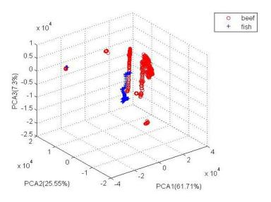
Figure 5. PCA plot of odor of both rotten beef with fresh fish and rotten fish with fresh beef.
