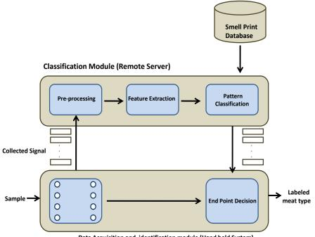
**Figure 1.** The overall block diagram of the electronic nose for the identification of spoiled meat.
