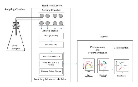
Figure 2. Electronic nose system.
