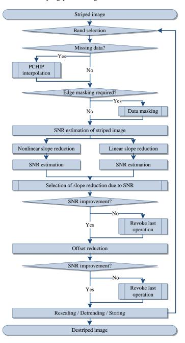
Figure 4. The destriping processing chain of the 'ROME' framework.
