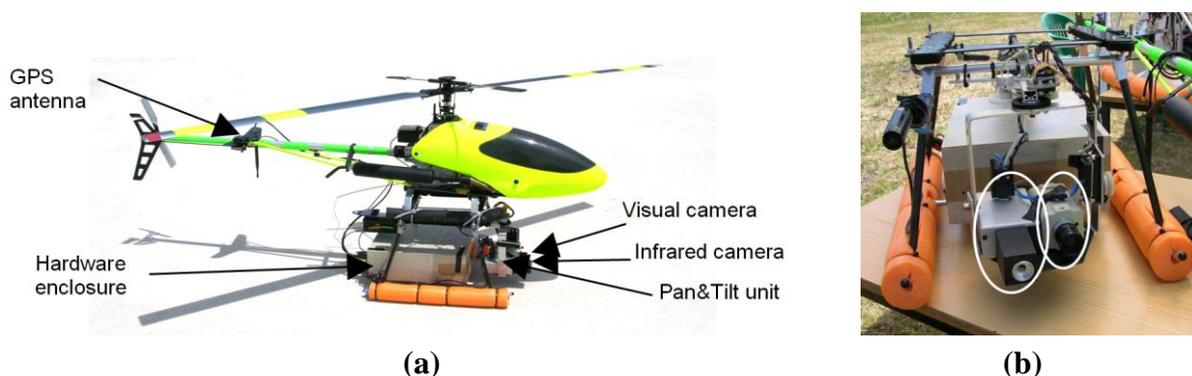
**Figure 4.** Diagram of the proposed forest-fire measurement system.
