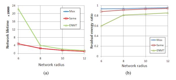
Different from the simulations in Figure 6, we change the maximum transmission range to 4 and 2 from inner group to outer group. Figure 7 shows the network lifetime and residual energy ratio with different algorithms. Obviously, the ENMT algorithm also performs better than the other two algorithms both in terms of network lifetime and residual energy ratio.
