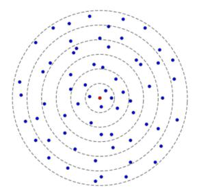
As shown in Figure 2, we partition the whole region with radius *R* into *m* adjacent concentric parts called coronas like in [8]. The width of each corona is *d* and  $C_i$  denotes the *i*th corona. The corona  $C_i$  includes all nodes whose distances to the sink nodes are between (i - 1) d and *id*. Therefore:
