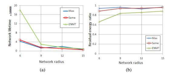
Different from previous simulations, the maximum transmission range is set to 4, 3 and 2 from inner group to outer group. Figure 9 shows the network lifetime and residual energy ratio with different algorithms. Obviously, the ENMT algorithm also outperforms than the other two algorithms both in network lifetime and residual energy ratio.
