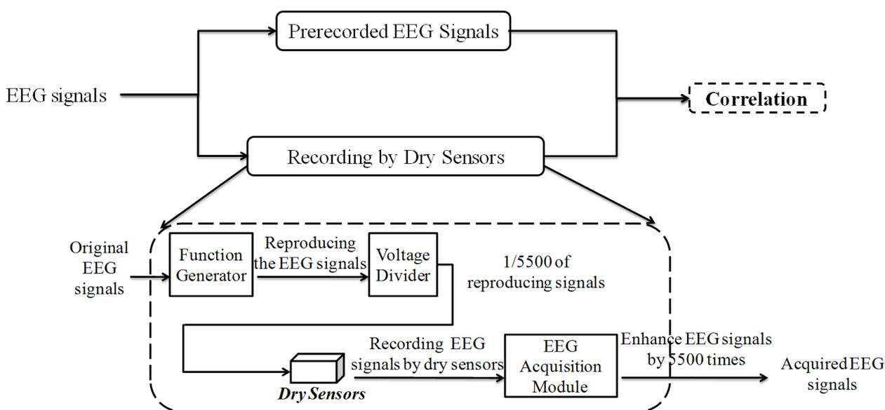
**Figure 8.** Prerecorded EEG and corresponding signals recorded by the dry EEG sensor.
