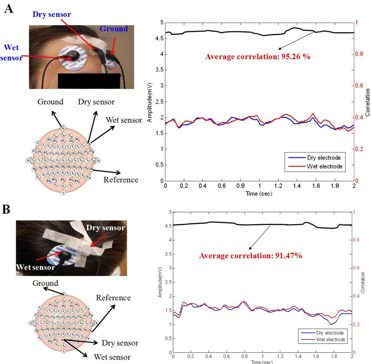
**Figure 10.** Signal comparison, as recorded by the wet electrodes and the proposed dry sensors. (A) The EOG measurements on a forehead site and (B) eye-blink signals on a forehead site are shown.
