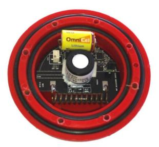
**Figure 2.** The sensor unit for temperature and oxygen consecration measurements within the protective housing.
