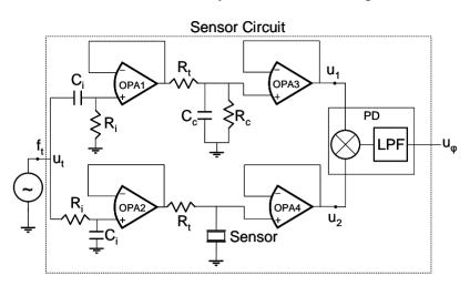
Figure 4. Schematics of the interface system for the sensor phase characterization.
