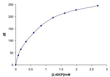
As the concentration of the pollutant increases, the change in fluorescence intensity gradually becomes small indicating that the change observed is due to interaction between the cyclodextrin and the pollutant. As the concentration increases the cyclodextrin cavities get saturated and therefore no more change in fluorescence is observed.
