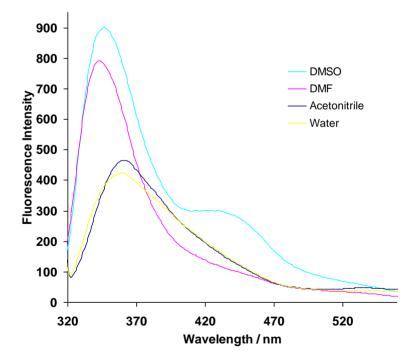
The fluorescence intensity of the polymer is greatly enhanced in DMSO and in DMF as compared to acetonitrile and water. A blue shift is also observed with the former solvents with the fluorescence being shifted from around 370 nm for acetonitrile and water to around 350 nm for DMSO and DMF. The polarity of the solvents used is in the order  $H_2O > DMSO > CH_3CN > DMF$ . Since there is no
