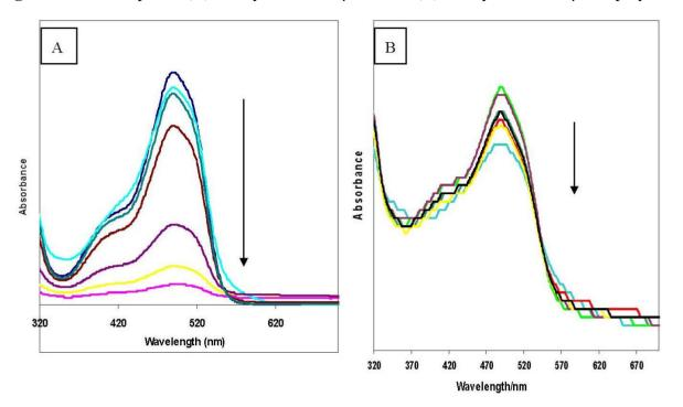
**Figure 1.** Effect of pH on (**A**) azo dye modified  $\beta$ -CD and (**B**) azo dye modified  $\beta$ -CD polymer.
