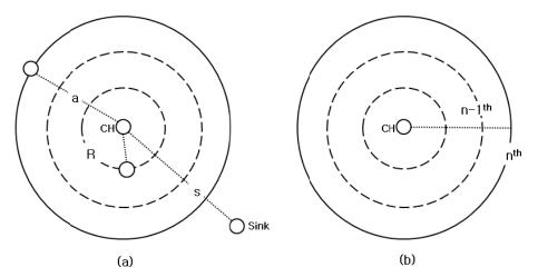
The total number of cluster-heads in a network is defined as m, therefore the area of the sensor networks is the same as the total area of local clusters which can be calculated as  $a^2\pi \times m = A^2$ . From this, we can figure out the radius of a local cluster, 'a', as:
