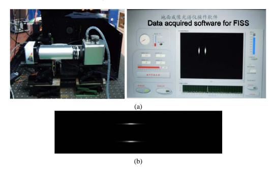
Due to the instability of the monochromator and the discrete spectra emitted from it, the spectral response curve of each channel is discrete and has a certain amount of noise. Hence, Gaussian fitting was used for the spectral curve of each channel. The center wavelength and spectral resolution of each channel were then calculated from the function. The Gaussian fitting function used in this paper was:
