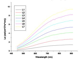
**Table 3.** Partial results of absolute radiometric calibration. (Aperture size, F/8; CCD cooling temperature, 10  $^{\circ}$ C; integration time, 30 ms).
