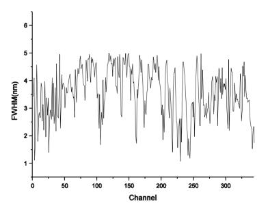
Figure 8. Spectral resolution for all 344 channels of the FISS system.
