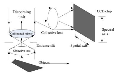
Figure 1. Basic principle of the FISS instrument.
