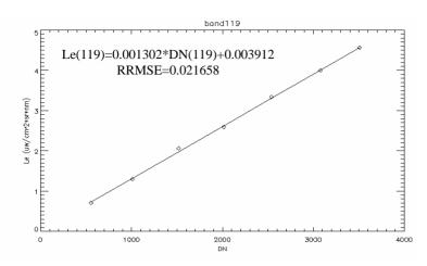
Figure 14. The FISS system radiometric calibration results of band 119.
