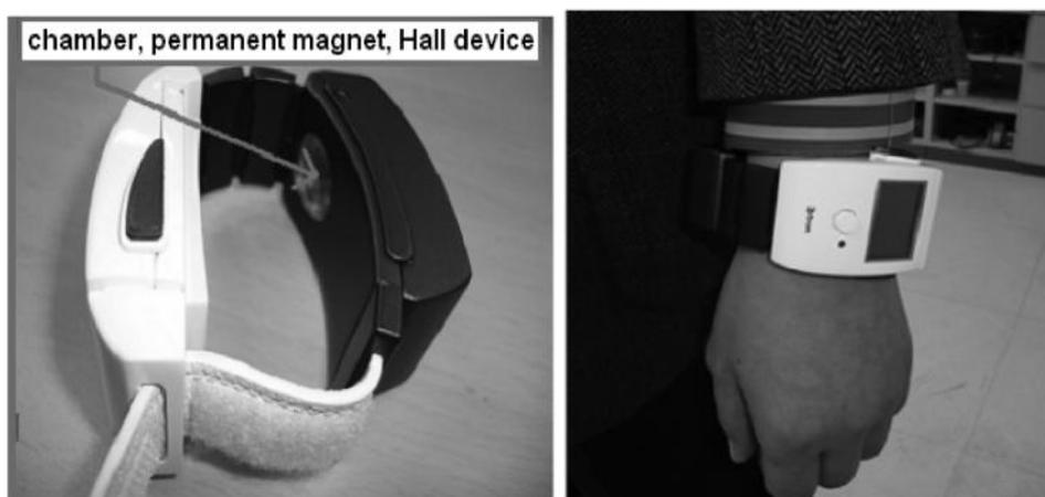
The first radial artery pulsometer we have developed is shown in Figure 5 and uses a Hall device to obtain the data. A permanent magnet and a Hall device placed inside an air bladder are arranged to safely contact the biggest pulse spot on the radial artery. The pulsometer weight has been reduced to about 80 g, including the battery. Our tests showed that the amount of electrical power provided by a lithium battery is less than 1.65 W (Output current 500 mA, 3.4 V) after wearing the pulsometer.
