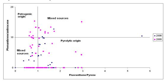
The percentage relationship between pyrolytic, petrogenic and other sources of PAH emissions (shown in Table 5), needed for assessing the origin of PAHs found in the runoff samples from Gdansk Airport, suggest that fuel combustion is the main source of PAH emissions.
