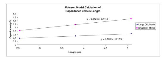
Given the Poisson model, along with qualitative experimental evidence, suggests a unique length extension  $\delta\lambda$  is required to correct for the extra fringe capacitance in coaxial cell type measurements, or TDR soil probes; therefore we propose a new variant for Equation 12, to allow for correction of the fringing field effects which is proposed herein as Equation 14.
