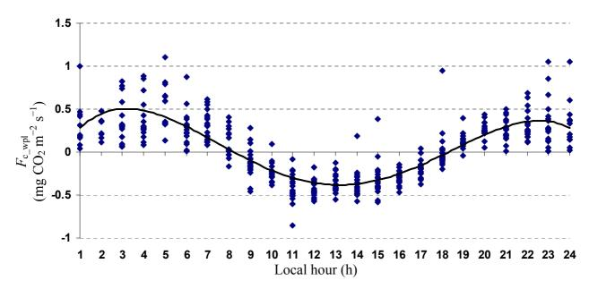
**Figure 5.** A quartic function fitted to  $F_{c_wpl}$  dataset for Yenicaga peatland in August of 2010:  $F_{c_wpl}$  (mg CO<sub>2</sub> m<sup>-2</sup> s<sup>-1</sup>) = 0.3242 h - 0.0696 h<sup>2</sup> ± 0.0044 h<sup>3</sup> - 9 × 10<sup>-5</sup> h<sup>4</sup>; ( $R^2_{adj} = 0.5963$ ; SE = 0.1957; n = 620; P < 0.001).
