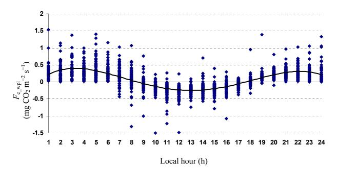
**Figure 4.** A quartic function fitted to  $F_{c_wpl}$  dataset for Yenicaga peatland in July of 2010:  $F_{c_wpl} (mg \text{ CO}_2 \text{ m}^{-2} \text{ s}^{-1}) = 0.3575 \text{ h} - 0.077 \text{ h}^2 \pm 0.0049 \text{ h}^3 - 9 \times 10^{-5} \text{ h}^4$ ;  $(R^2_{adj} = 0.7087; \text{ SE} = 0.1905; n = 412; P < 0.001)$ .
