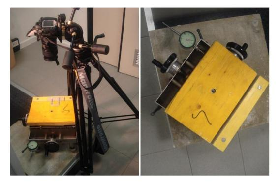
Figure 3. The sledge used to check the accuracy of the image-based tool.
