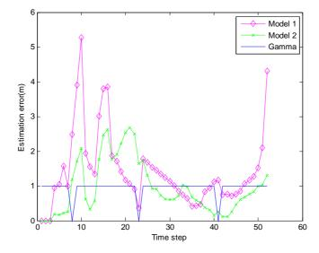
**Figure 11.** Estimation error of different filters with IDGSS under packet arrival rate p = 0.90.
