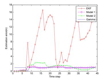
**Figure 10.** Estimation error of different filters with IDGSS under packet arrival rate p = 0.95.
