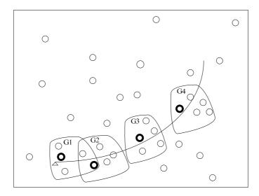
**Remark 3**: we use dynamic grouping idea and firstly awake M sensor nodes in order to increase real-time performance of target tracking, and adopt the changed sampling intervals during target tracking in order to save energy consumption under the satisfactory estimation accuracy.
