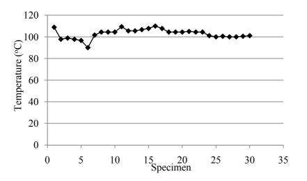
Thus, temperature sensors are not viewed as effective indicators of abrasive life and loading formation, however, they were found to be effective in helping establish high temperature limits in order to avoid burning the wood surface and / or belt damage.
