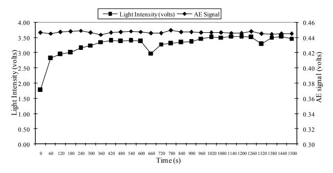
Figure 6 showed that the contact resonant AE sensor was able to measure belt wear with the appropriate location even for the belt speeds experienced during machining (43.33 ft/s–3.62 m/s).
