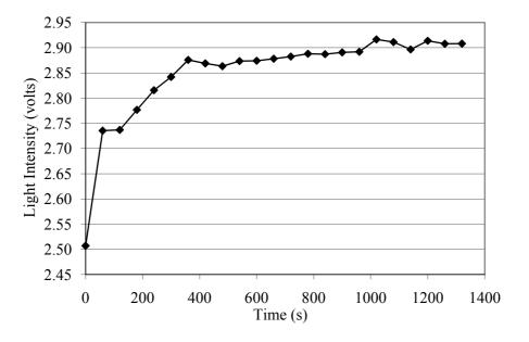
**Figure 3.** Wenglor® optical sensor signal after cleaning with CO<sub>2</sub> flakes every 400 seconds during abrasive machining.
