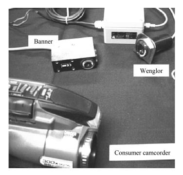
Different types of sensors were studied and analyzed in order to identify the best combination of sensors for monitoring loading and temperature, thus, optical sensors (color and gray scale) were used to monitor abrasive loading and IR thermometers were used to monitor temperature.
