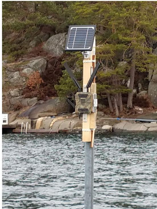
**Figure 2.** Time-lapse camera used in Lyngør. It consisted of a Bushwhacker Camo 4G camera connected to a solar panel for power supply. The same setup is used in Østre Bolæren. Photo credit: Elsa van Meurs.
