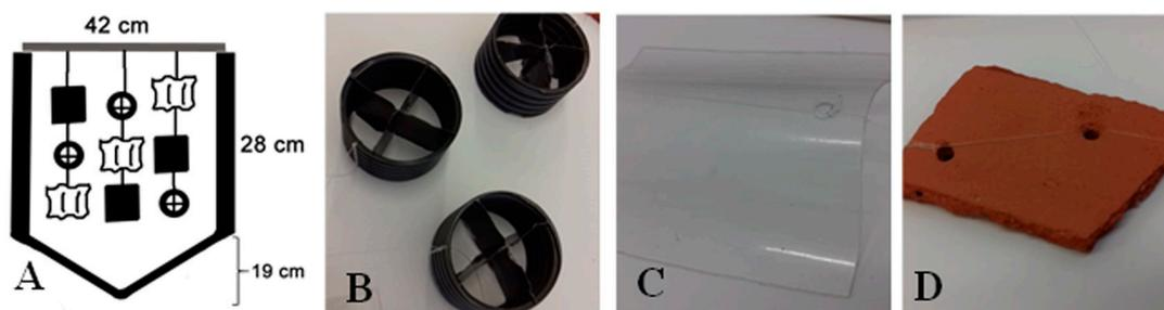
**Figure 1.** Illustration of the different substrates used for the settlement trials, including (A) Design and dimensions of the rearing tanks and the substrate structures within (B) PVC roll; (C) Wavy PVC plaque and (D) Tile fragment.
