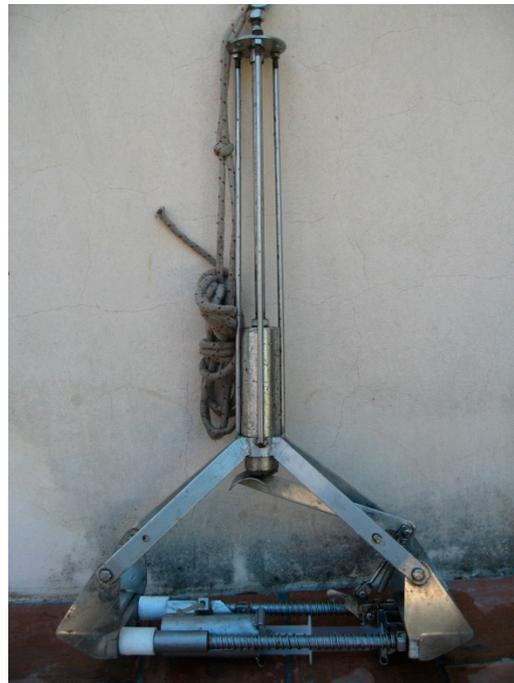
**Figure 5.** Horizontal coring instrument for collecting 60 mL of surface sediment (3–4 cm thick). After positioning the instrument's base on the bottom, sending the messenger (vertically arranged metal block) triggers the spring that drags the syringe along the horizontal path at the instrument's base, collecting the sediment material.
