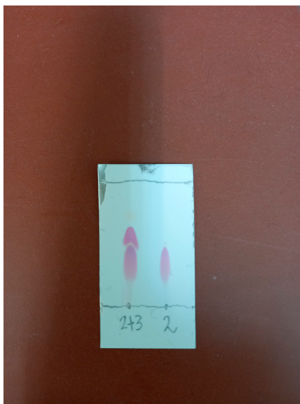
Figure S12: Analytical TLC (7 % MeOH/CH 2 Cl 2 ); left—mixture of compounds (2+3); right—compound 2 after purification by preparative TLC (7 % MeOH/CH 2 Cl 2 ); the spots were visualised by exposing the analy. plate to UV irradiation (UV lamp, 254 nm, 4 min.)
