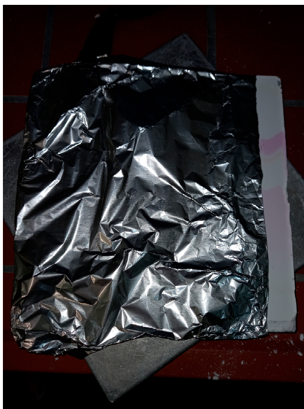
Figure S11: Preparative TLC (7 % MeOH/CH 2 Cl 2 ) used for isolation of compounds from mixture 2+3 ; the stripes are located (visualized) by exposing the edge part of the plate to UV irradiation (254 nm, 2-3 min)-the irradiated area becomes “dark pink” due to DAE unit cyclisation on spot. The unirradiated stripes of SiO 2 are separated according to “dark pink” regions.
