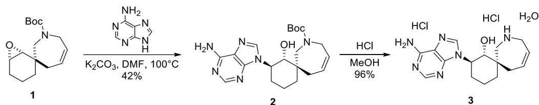
**Scheme 1.** The opening of epoxide **1** with adenine and synthesis of ((1*RS*,2*RS*,6*RS*)-2-(6-Amino-9*H*-purin-9-yl)-8-azaspiro[5.6]dodec-10-en-1-ol dihydrochloride (**3**).
