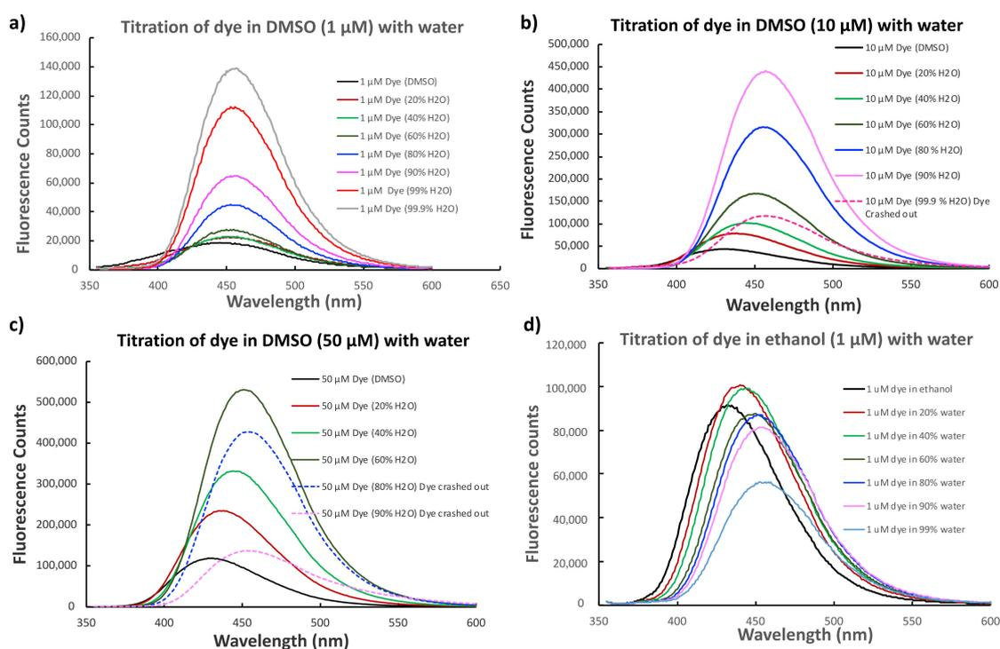
**Figure 2.** Changes in fluorescence intensity of 4-phenyl-1,8-naphthalimide in DMSO and ethanol upon addition of water. (a). 1  $\mu\text{M}$  dye in DMSO, (b). 10  $\mu\text{M}$  dye in DMSO, (c). 50  $\mu\text{M}$  dye in DMSO, and (d). 1  $\mu\text{M}$  dye in ethanol.
