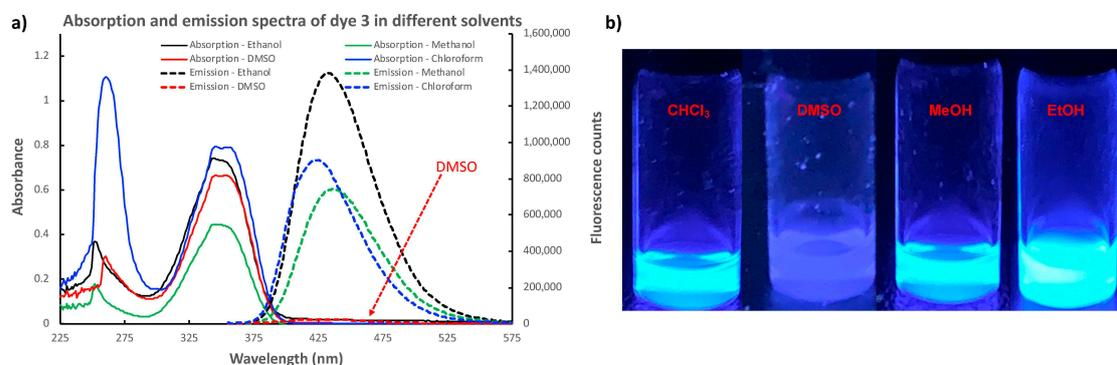
**Figure 1.** Photophysical properties of 4-phenyl-1,8-naphthalimide. (a). Absorption and emission profiles of 4-phenyl-1,8-naphthalimide in chloroform, DMSO, methanol and ethanol. Solid lines: absorption spectra recorded at 100  $\mu\text{M}$ ; dotted line: emission spectra recorded at 10  $\mu\text{M}$ , excited at 345 nm; (b). pictures of 4-phenyl-1,8-naphthalimide in chloroform, DMSO, methanol and ethanol, excited with a handheld UV lamp (360 nm).
