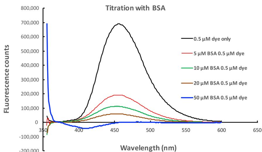
**Figure 5.** Quenching of 4-phenyl-1,8-naphthalimide by BSA. The fluorescence spectra with BSA samples were derived after subtraction of that of BSA of corresponding concentrations.
