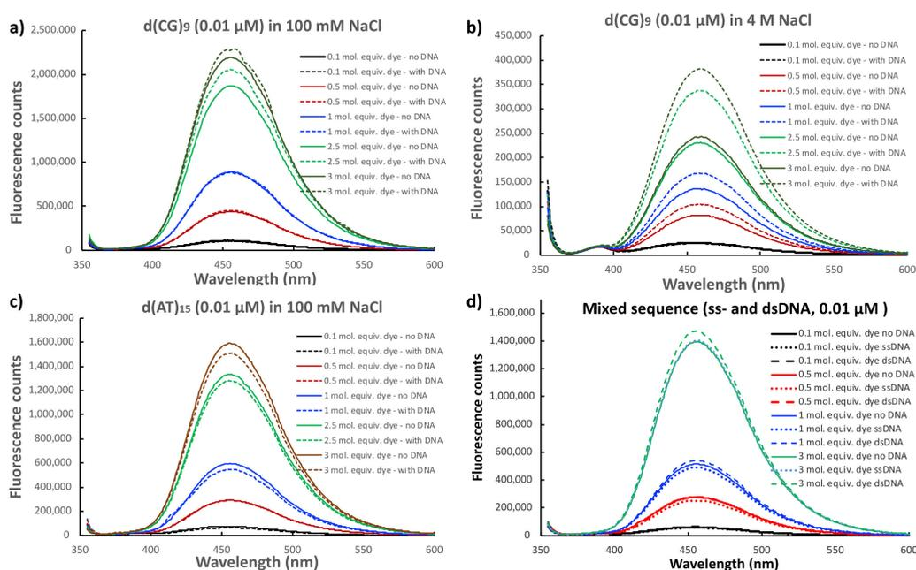
**Figure 3.** Fluorescence profiles of 4-phenyl-1,8-naphthalimide in the presence of DNA. (a) d(CG)<sub>9</sub> in 100 mM NaCl; (b) d(CG)<sub>9</sub> in 4 M NaCl; (c) d(AT)<sub>15</sub> in 100 mM NaCl; and (d) mixed sequence ss- and ds-21-mer, d(TGGTATATCTCCTTCTTAAAG).
