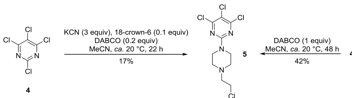
**Scheme 3.** Synthesis of 2,4,5-trichloro-6-[4-(2-chloroethyl)piperazin-1-yl]pyrimidine (5).
