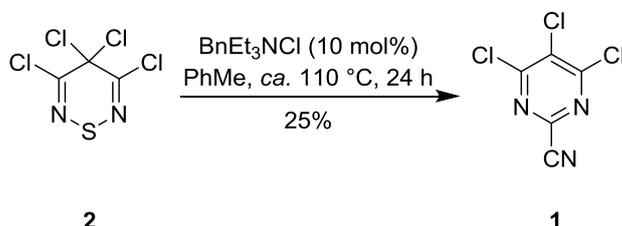
**Scheme 1.** Isolation of trichloropyrimidine **1** from 3,4,4,5-tetrachloro-4*H*-1,2,6-thiadiazine (**2**).
