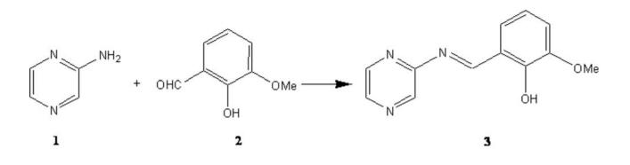
A mixture of 2-amino pyrazine 1 (0.95 g, 10.00 mmol), o-vanillin (2-hydroxy-3-methoxy benzaldehyde) 2 (1.52 g, 10.00 mmol) and anhydrous sodium sulfate (3.00 g) in dry dichloromethane (40.00 mL) was stirred at room temperature for five hours. The suspension was filtered and washed with CH<sub>2</sub>Cl<sub>2</sub>. The solvent was evaporated under reduced pressure and imine 3 was formed as a red solid which was recrystalized from methanol (1.90 g, 83%).
