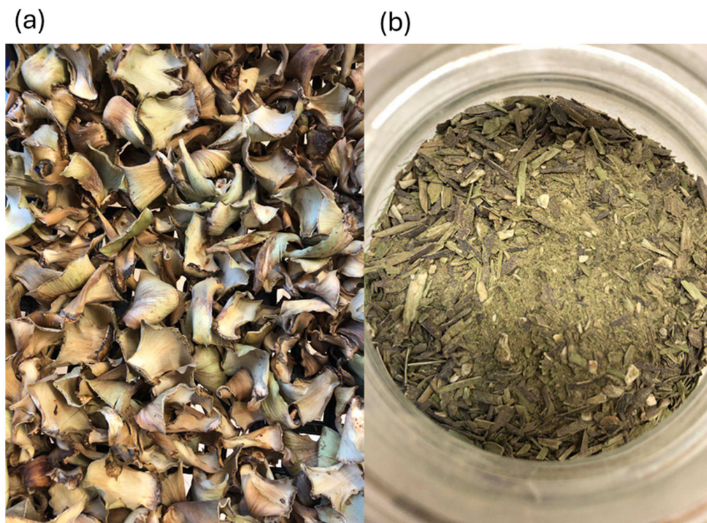
Figure 5. Representative images of artichoke by-product (ABP) bracts at different processing stages: (a) freshly dried bracts after oven-drying at 40 °C; (b) ground bracts after milling and sieving (300–600 µm particle size).
