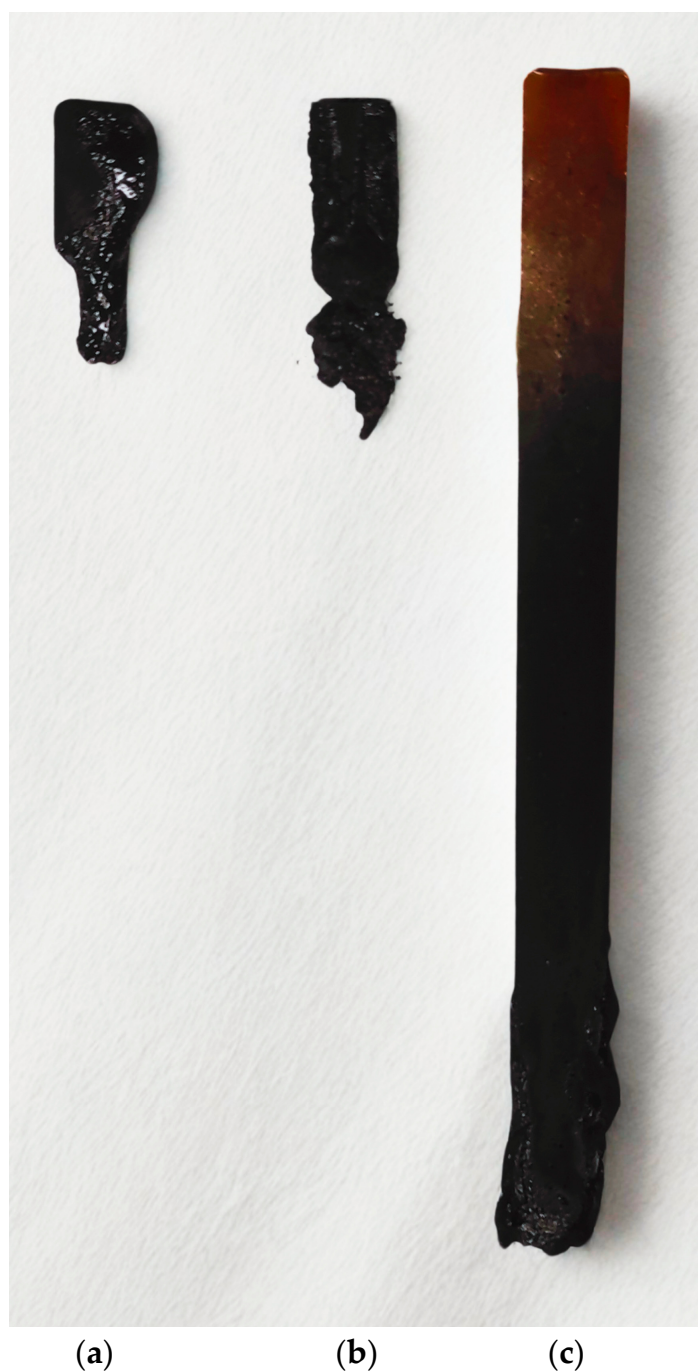
Figure 2. The samples tested after the UL-94 vertical burning tests: (a) EP0, (b) EP10TEP, (c) EP30TEP.
