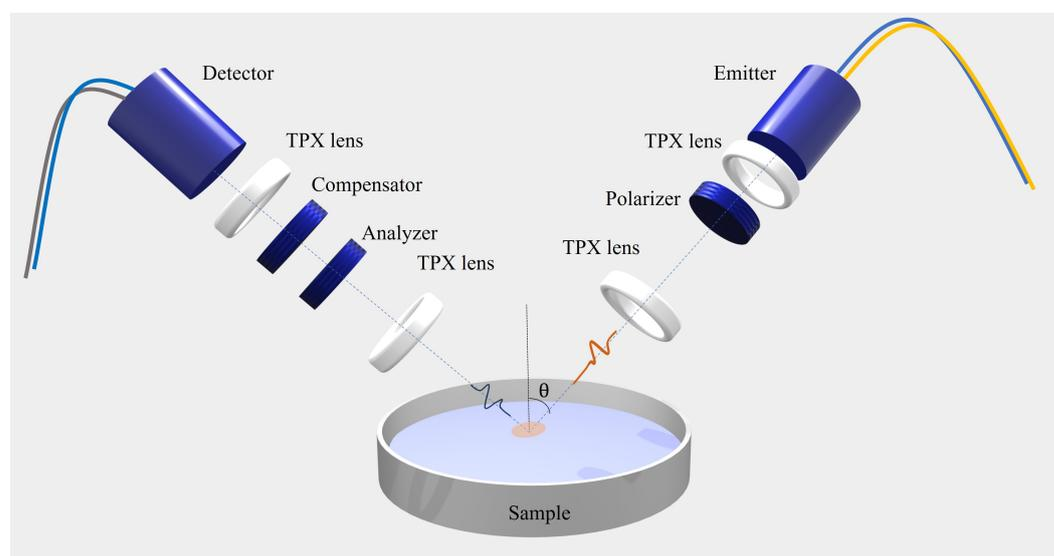
**Figure 4.** Sketch of the opto-mechanical setup depicting the customized fiber-coupled THz TDSE.
