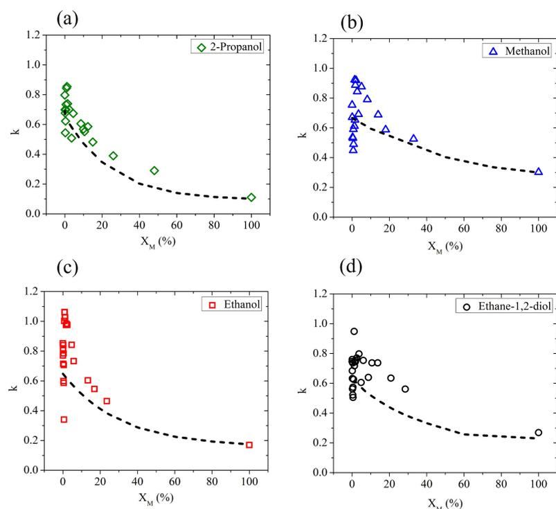
**Figure 2.** The experimental values (averaged over four different frequency points: 0.3, 0.6, 0.9, and 1.2 THz) of  $k$  in aqueous binary mixtures based on (a) 2-propanol, (b) methanol, (c) ethanol, and (d) ethane-1,2-diol measured as a function of the solute molar fraction (solid points). Dot-dashed lines describe the prediction of the effective Debye model.
