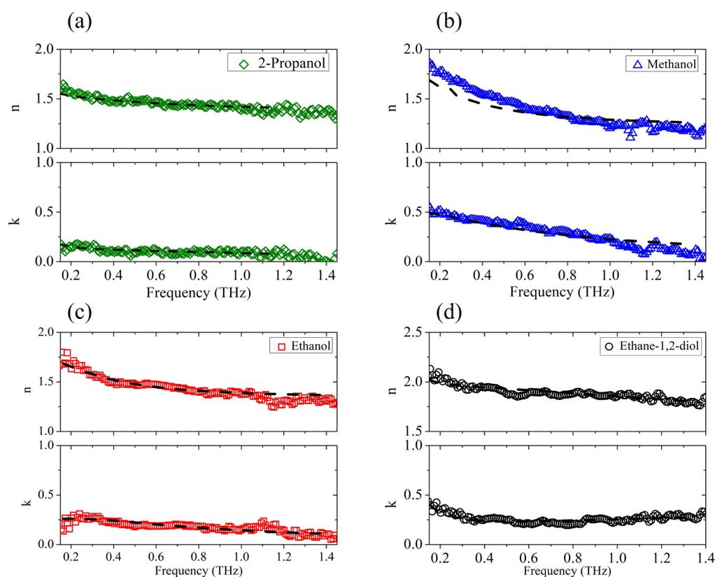
**Figure 1.** The experimental complex refractive index  $n - ik$  vs. frequency (solid points) for (a) 2-propanol, (b) methanol, (c) ethanol, and (d) ethane-1,2-diol, and its fit (dot-dashed lines) to the generalized Debye model.
