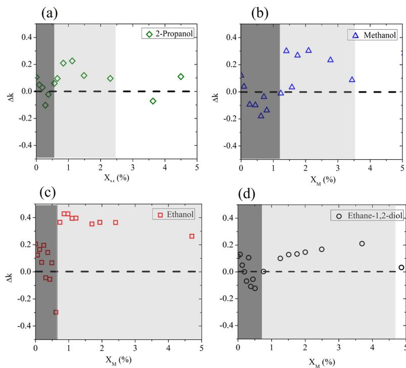
**Figure 3.** Deviation  $\Delta k$  (frequency averaged) between the experimental data and the prediction of the Debye model for aqueous binary mixtures based on (a) 2-propanol, (b) methanol, (c) ethanol, and (d) ethane-1,2-diol, measured at a low solute molar fraction. The dashed horizontal line marks the difference with the expected Debye behavior.
