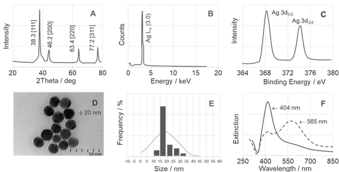
**Figure 2.** Surface analysis of AgNPs, with XRD–(A), EDS–(B), XPS–(C), TEM–(D), DLS–(E), and UV-VIS–(F).
