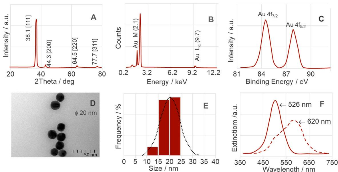
**Figure 3.** Surface analysis of AuNPs, with XRD–(A), EDS–(B), XPS–(C), TEM–(D), DLS–(E), and UV-VIS–(F).
