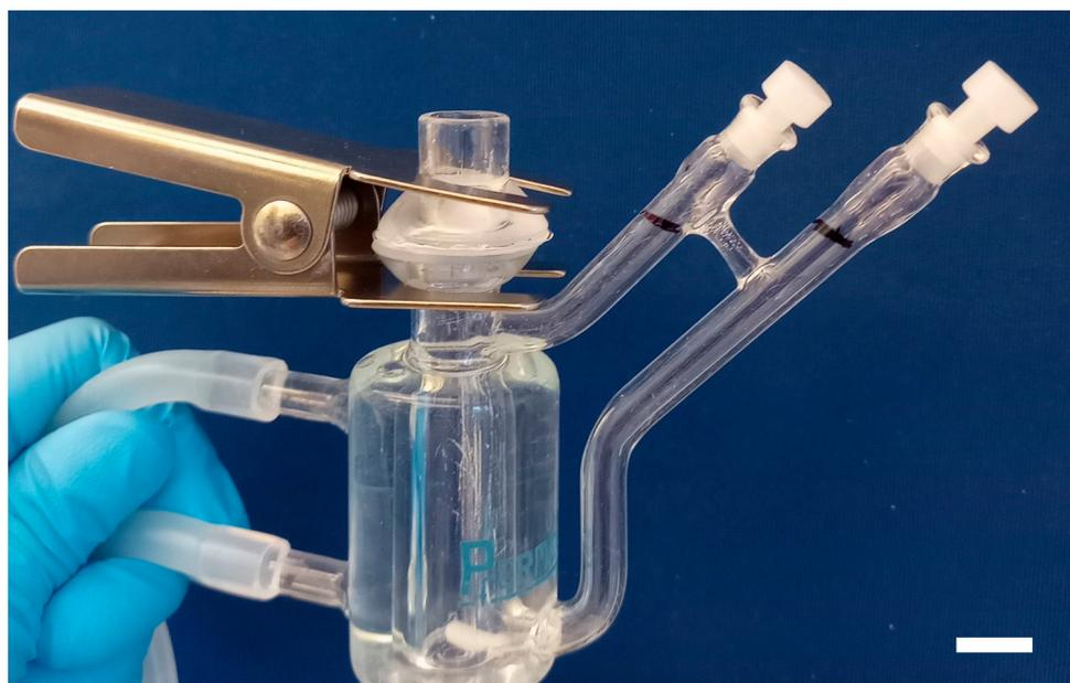
**Figure 5.** Franz Cell (PermeGear) used in the studies on NPY release. Scale bar, 10 mm.
