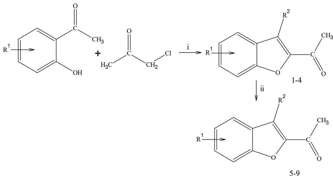
Reagents and conditions: i:  $K_2CO_3$ , heating; ii: carbon tetrachloride ( $CCl_4$ ), N-bromosuccinimide (NBS), benzoyl peroxide, heating.
