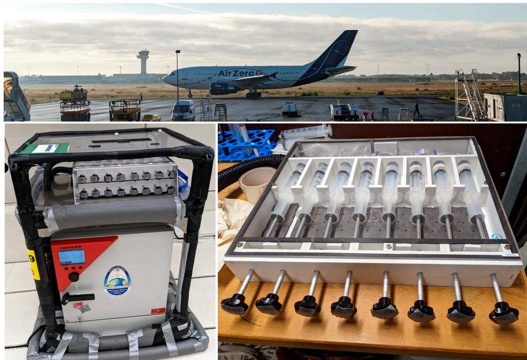
**Figure 2.** Impressions of the 41st DLR parabolic flight campaign in September 2023, Bordeaux, France. The Airbus A310 Zero G aircraft of Novespace (**top**), the flight rack of the “Thyroid” mission (**bottom left**) and its RNAlater injection system (**bottom right**) are shown.
