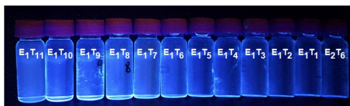
**Figure 3.** The photographs of  $E_1T_1$  to  $E_1T_{11}$  and  $E_2T_6$  in ethanol solutions under 365 nm UV light.
