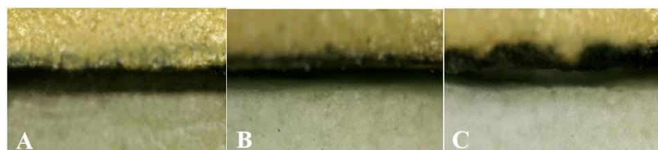
**Figure 9.** Marginal fit of PFM dental restoration after final glazing procedure at  $\times 300$  magnification (A) casting, (B) milling, (C) SLM.
