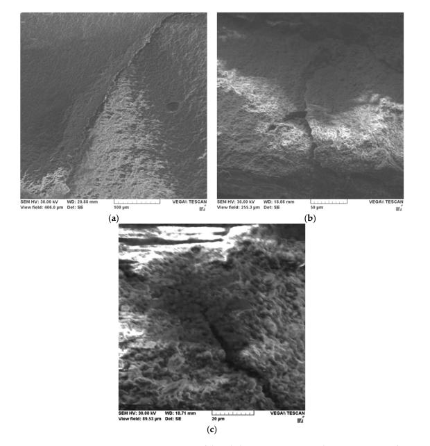
**Figure 3.** SEM microscopies of the Filtek Supreme XT-2 sample at various magnification powers:  $700 \times$  (**a**),  $1100 \times$  (**b**) and  $3200 \times$  (**c**).
