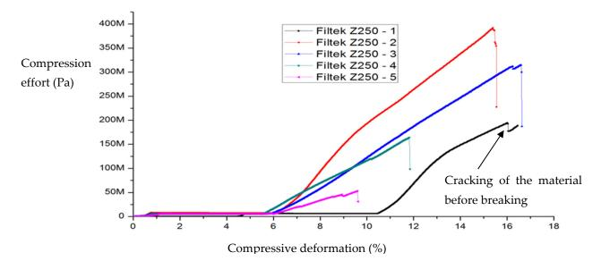
Figure 2. Variation of compressive strain with compressive stress for Filtek Z250 composite specimens.
