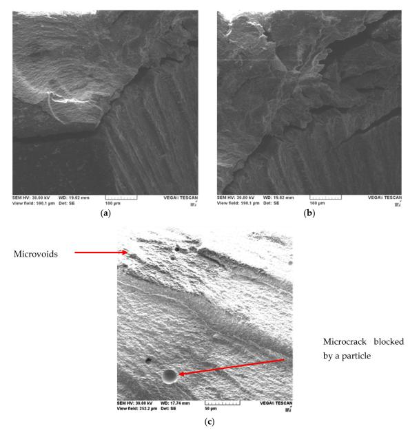
**Figure 5.** SEM microscopy of the Filtek Z250—1 sample at various magnifications  $500 \times (\mathbf{a}, \mathbf{b})$ ,  $1150 \times (\mathbf{c})$  showing some micro voids resulting from the pulling out of the filler particles.
