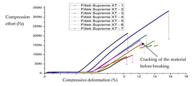
Figure 1. Variation of compressive strain with compressive stress for Filtek Supreme XT composite specimens.
