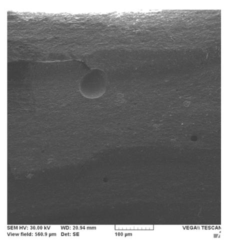
**Figure 6.** SEM microscopy of Filtek Z250-4 sample with microcrack blocked by a micrometer particle and areas with effective micro filler pull-outs.
