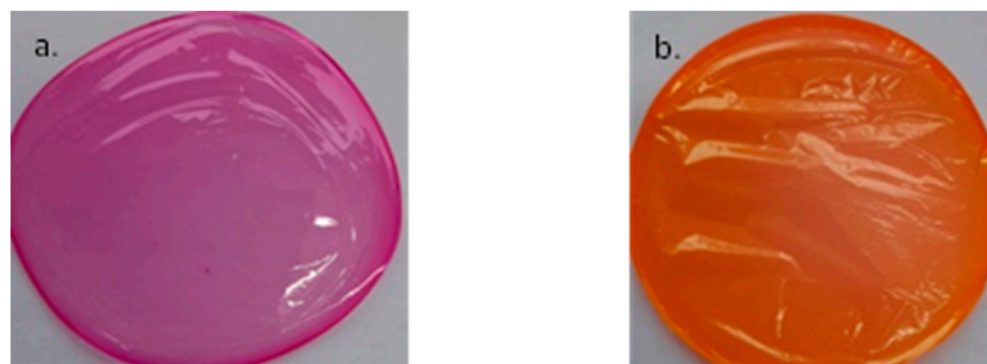
Figure 2. Photo of chitosan film (a) with 5% addition of I and (b) with 5% addition of H dyes.
