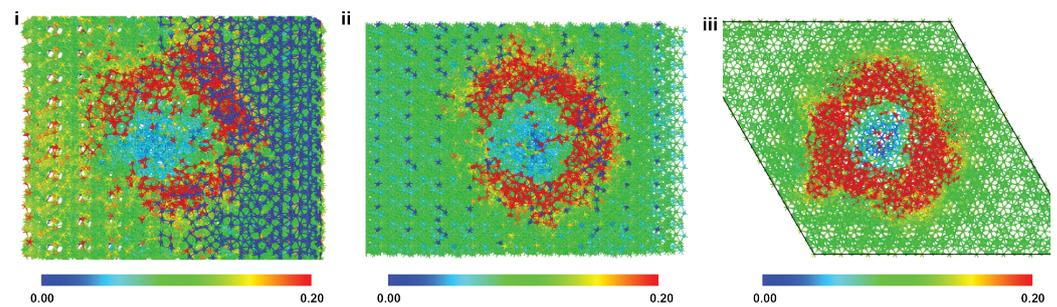
**Figure 7.** Atomic snapshots of HAP models containing 30 Å pores at the inception of compressive failure for X (i), Y (ii), and Z (iii) loading. Atoms are colored according to the atomic shear strain. X and Y loading images are viewed in the X-Y plane, whereas the Z loading image is in the Y-Z plane.
