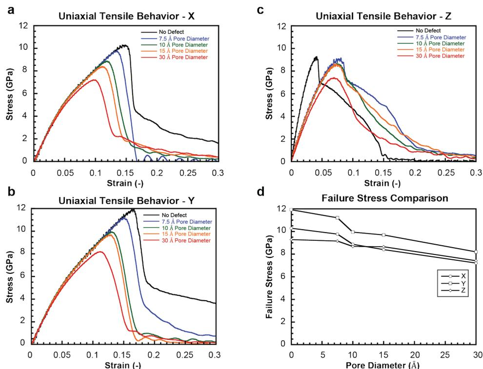
**Figure 1.** Effect of pore inclusion on HAP tensile mechanical response. (a–c) X, Y, and Z direction stress–strain curves for monocrystalline HAP with and without pores of different sizes, respectively. (d) Measured failure stress for each loading direction as a function of pore size.
