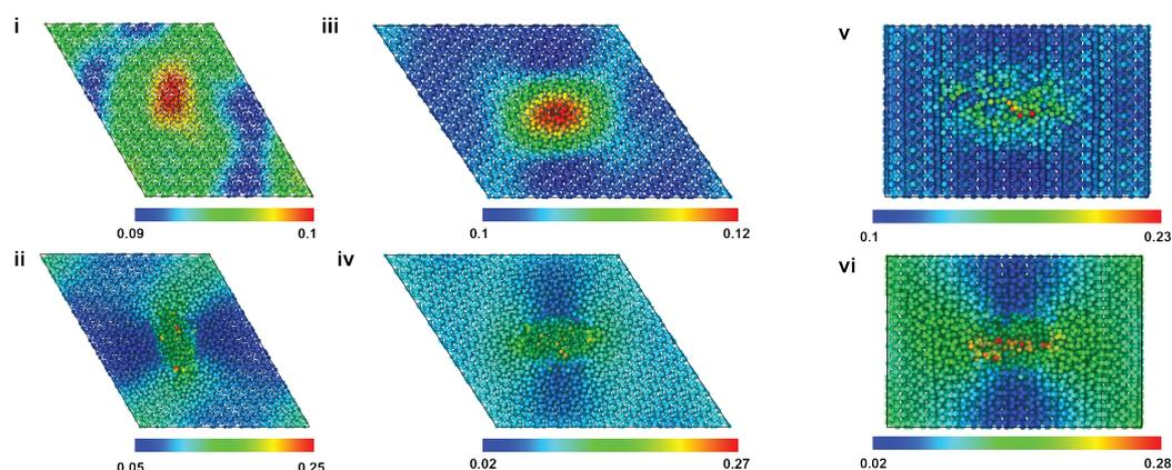
**Figure 5.** Atomic snapshots of HAP models at the inception of compressive failure for 7.5 Å (top row) and 30 Å (bottom row) pores, for X (i,ii), Y (iii,iv), and Z (v,vi) loading. Atoms are colored according to the von Mises shear strain. The view of the snapshots for X and Y loading is the X-Y plane, and it is the Y-Z plane for the Z loading.
