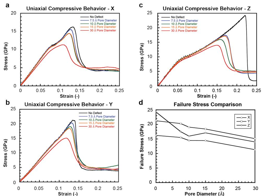
**Figure 4.** Effect of pore inclusion on HAP compressive mechanical response. (a–c) X, Y, and Z direction stress–strain curves for monocrystalline HAP with and without pores, respectively. (d) Measured failure stress for each loading direction as a function of pore size.
