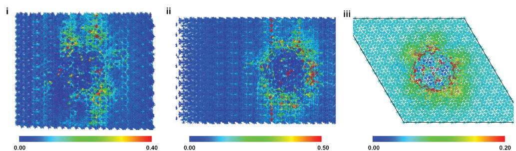
**Figure 3.** Atomic snapshots of HAP models containing 30 Å pores at the inception of tensile failure for X (i), Y (ii), and Z (iii) loading. Atoms are colored according to the atomic shear strain. X and Y loading images are viewed in the X-Y plane, whereas the Z loading image is in the Y-Z plane.
