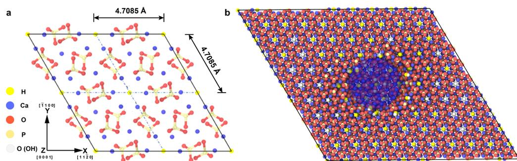
**Figure 8.** Simulated HAP domain. (a) The 44-atom HAP unit cell used as the base for replication. (b) Sectioned 44,000 atom HAP domain showing a 30 Å diameter pore at the center (shaded blue for clarity).
