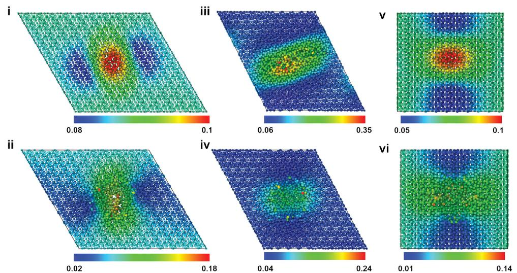
**Figure 2.** Atomic snapshots of HAP models at the inception of tensile failure for 7.5 Å (top row) and 30 Å (bottom row) pores, for X (i,ii), Y (iii,iv), and Z (v,vi) loading. Atoms are colored according to the von Mises strain. X and Y loading images are viewed in the X-Y plane, whereas the Z loading image is in the Y-Z plane.
