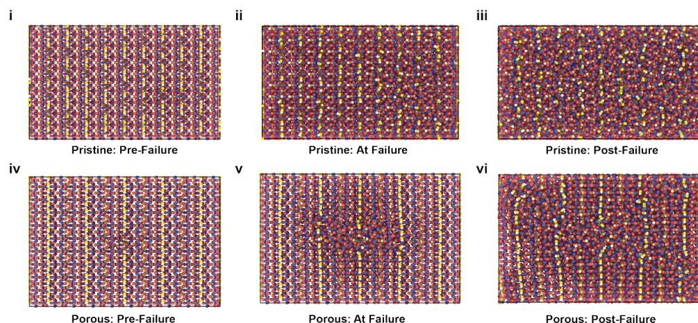
**Figure 6.** Atomic snapshots of the pristine HAP model (i–iii) and of the HAP model having a 7.5 Å pore (iv–vi) at various time-steps, i.e., before failure, at the inception of failure, and after failure under compressive loading in the Z direction. The view is in the Y-Z plane.
